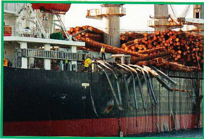
Close-up look of the damaged a massive vertical support beams bend like a matchstick
